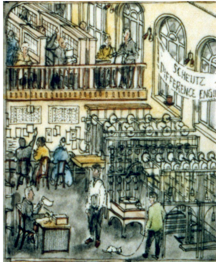
FIGURE 8: Computer Laboratory. The apparatus on the lower level is Scheutz's Difference Engine. On the upper level, Hollerith machines are shown.
