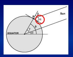
Angles used to calculate the latitude.
