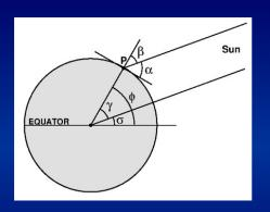
Angles used to calculate the latitude.
