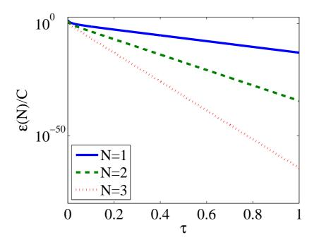
Figure 7.1: Error in the finite truncation of the diffusion equation, as a function of the truncation degree N, and as a function of elapsed time  $\tau$ .
