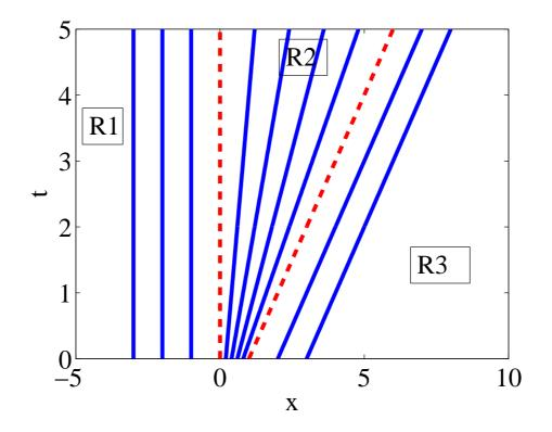
Figure 24.5: Characteristics of the Riemann problem with piecewise increasing initial data
