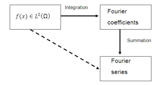
Fig. 4.2: The creation of a Fourier series from a generating function and the creation of functions from Fourier series are not **always** inverses: this is not a commutative diagram.
