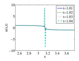
Figure 24.4: Failure of the numerical simulation of Burgers equation with  $u(x, t = 0) = \sin(x)$ , after t = 1.
