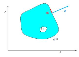
Figure 10.1: Gauss's theorem in the plane
