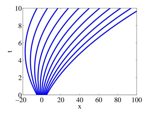
Figure 23.1: Characteristic curves for  $u_t + uu_x = 1$ , initial data u(x, t = 0) = x. The curves are given by Eq. (\*).
