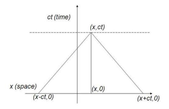
Figure 13.1: The domain of dependence for the wave equation
