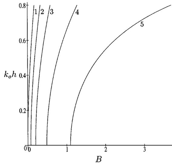
Figure 11 For a fixed angle  $\varphi$ , the existence of short-crested waves has been proved to the right of the curve corresponding to that angle. The curves represented here correspond to  $\varphi = 0$  (1),  $\varphi = \pi/8$  (2),  $\varphi = \pi/6$  (3),  $\varphi = \pi/5$  (4),  $\varphi = 2\pi/9$  (5).
