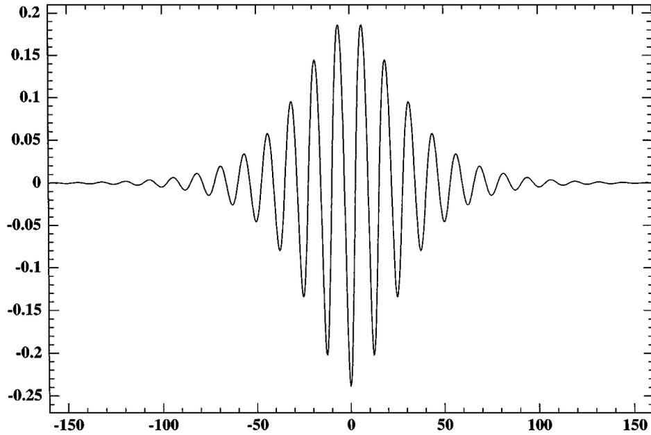
Figure 3 Profile of a solitary wave in deep water. The horizontal axis is  $X$  and the vertical axis is  $\eta$ .
