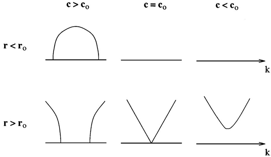
Figure 2 Bifurcation of periodic traveling waves near the critical point  $(k_o, c_o)$  when  $r \neq r_o$ . The case  $c > c_o$  was explained in Figure 1. For  $r < r_o$ , there are no periodic solutions with  $c < c_o$ . For  $r > r_o$ , the branches of periodic solutions coalesce at  $c = c_o$  and become a detached branch for  $c < c_o$ . These new periodic solutions exist only at finite amplitude.
