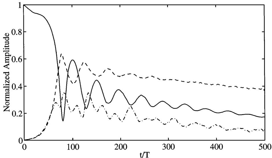
Figure 6 Time histories of the amplitude of the fundamental, subharmonic, and superharmonic modes ( $p = \frac{1}{3}$ ) for an evolving perturbed train of Stokes waves of initial steepness  $\epsilon = 0.20$ , wavelength  $L = 10$  cm, and fundamental period  $T$ .
