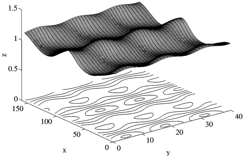
*Figure 7* 3D wave pattern that has evolved from a uniform Stokes wave train ( $\epsilon = 0.23$ ) by instability of class II ( $m = 1$ ) with  $p = \frac{1}{2}$  and  $q = \frac{3}{2}$ . The waves are propagating from right to left. The horseshoe patterns are in their phase of growth and have their wave fronts oriented forward. Drawing by C Skandrani (1997).
