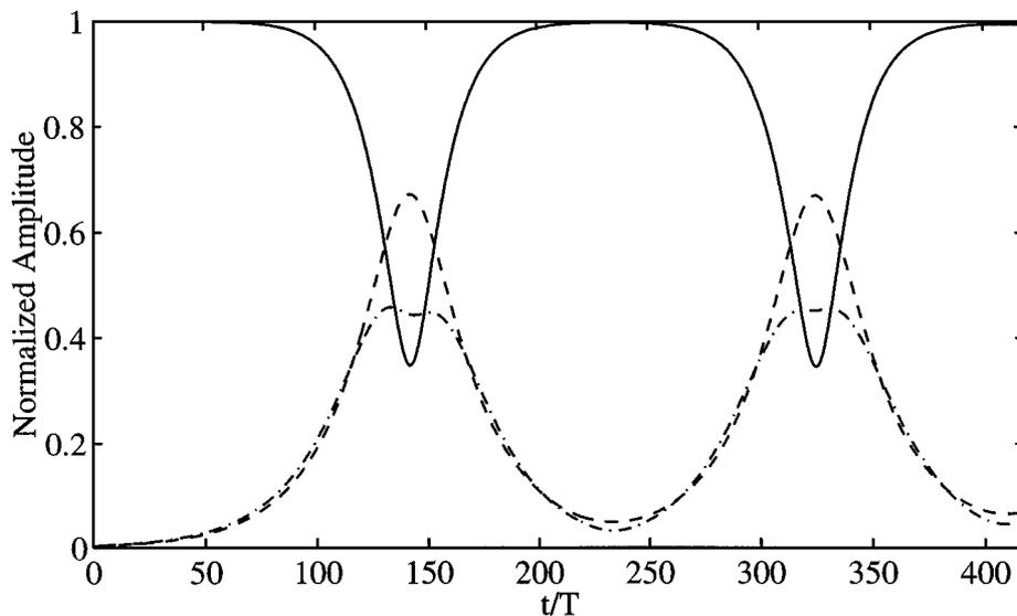
Figure 5 Time histories of the amplitude of the fundamental, subharmonic, and superharmonic modes ( $p = \frac{2}{3}$ ) for an evolving perturbed Stokes wave of initial steepness  $\epsilon = 0.13$  and fundamental period  $T$ .
