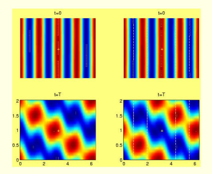
Initial and final fields for two four-day integrations. Initial fields differ only in the sign of the small perturbation. Drastically different patterns can result from states which are initially very similar!
