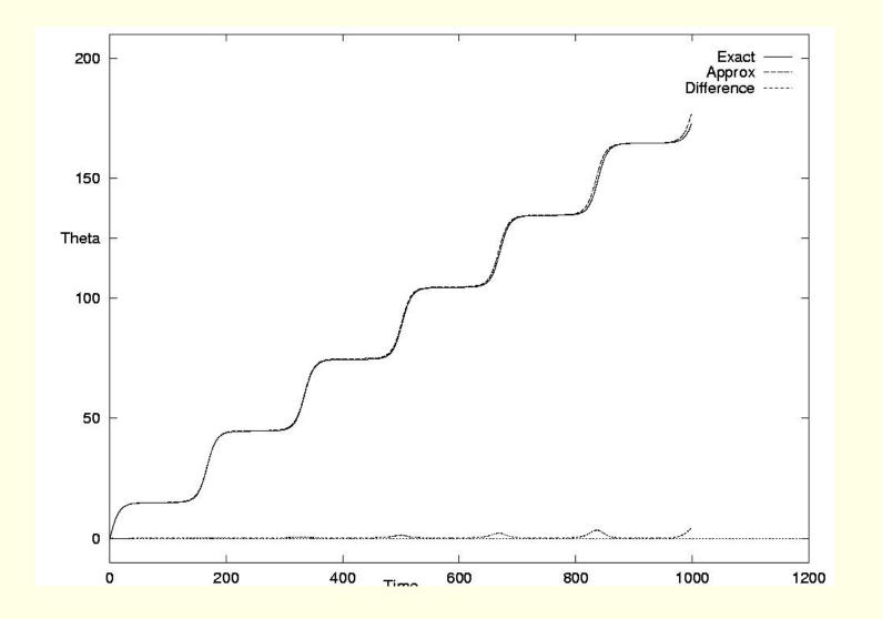
Azimuth for 'exact' and 'approximate' solutions. Difference plotted as dotted line.
