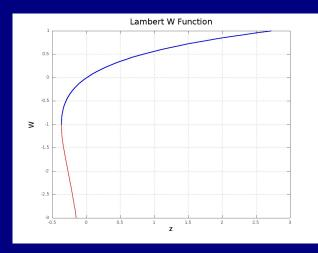
**Figure :** Lambert W-function w = W(z). The inverse of  $z = w \exp(w)$ .
