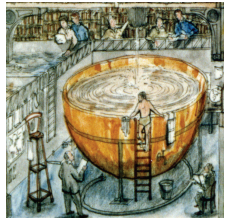
Figure 9. A large hemispheric bowl spinning on a turntable, for geophysical experiments. The figure standing below the tank is Sir G. I. Taylor. More water tanks are seen to the left.
